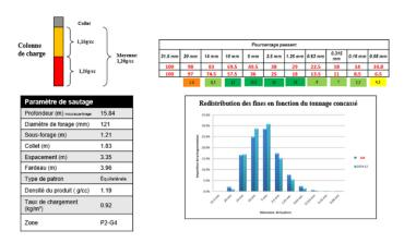
Figure 2: Parameters for blast no. 2014-12
